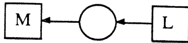
Figure B.2.7: An acquired lock resource and a request for a message resource.
