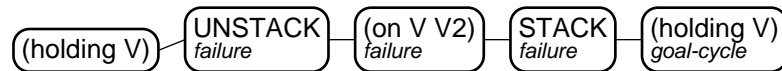
Figure 7: The PSG subgraph corresponding to the proof that UNSTACK fails to achieve holding.
