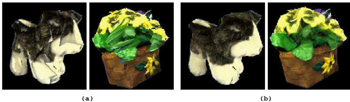
Figure 10 (a) The result of combining three views by repeatedly rendering the view-based meshes from the viewpoint of the virtual camera as described in Section 4.1. (b) Using the weights and soft z-buffering described in Section 4.2 produces a much better result.
