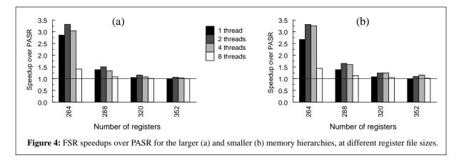
registers and 4 idle contexts (4 threads), FSR outperformed PASR by 8%, averaged over all applications. With only 288 or 264 registers, FSR's advantage grew to 34% and 205%, and with 6 idle contexts (and 320 registers) to 15%. Taking both factors into account (288/264 registers, 6 idle contexts), FSR outperformed PASR by 51%/232%. Only when all contexts were active were FSR and PASR comparable; in this case the architectural state for all threads is resident in both schemes.
