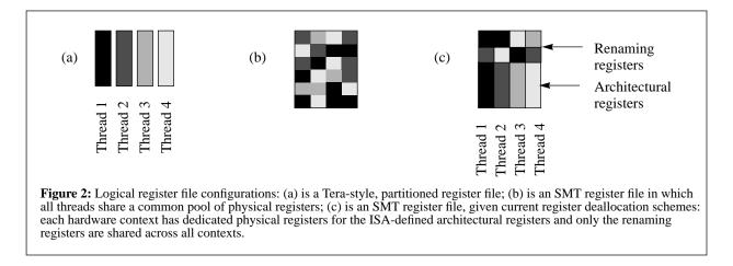
scheme to multiple contexts. Threads name architectural registers from their own context, and the renaming hardware maps these thread-private, architectural registers to the pool of threadindependent physical registers. Register renaming thus provides a transparent mechanism for sharing the register pool.
