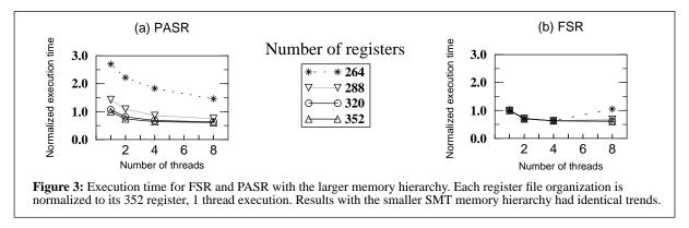
The speedups in Figure 4 show that FSR equals or surpasses PASR for all register file sizes and numbers of threads. FSR provides the greatest benefits when it has more registers to share (several idle contexts) and PASR has fewer (small register files). For example, with 320
