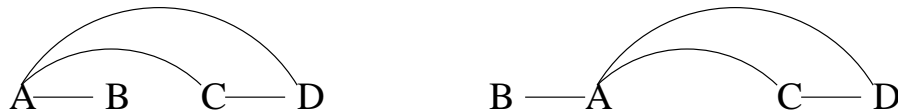
Figure 1: An example of an under-constrained ordering (Probe B can be placed on either side of probe A ). A line between two probes indicates a measurement between the probes.
