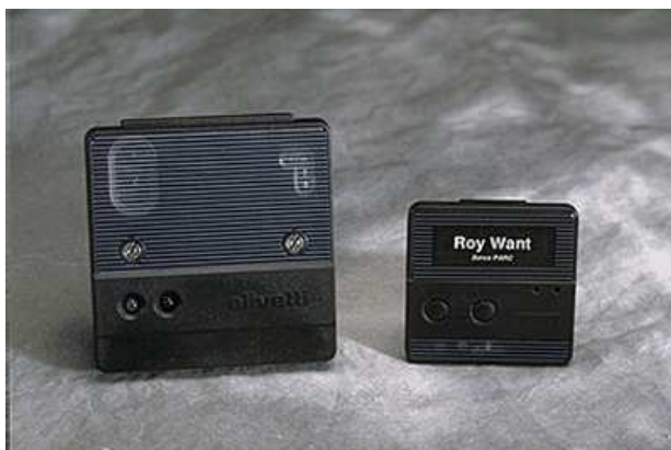
Figure 5: Olivetti Active Badge (right) and a base station (left) used in the system's infrastructure.
