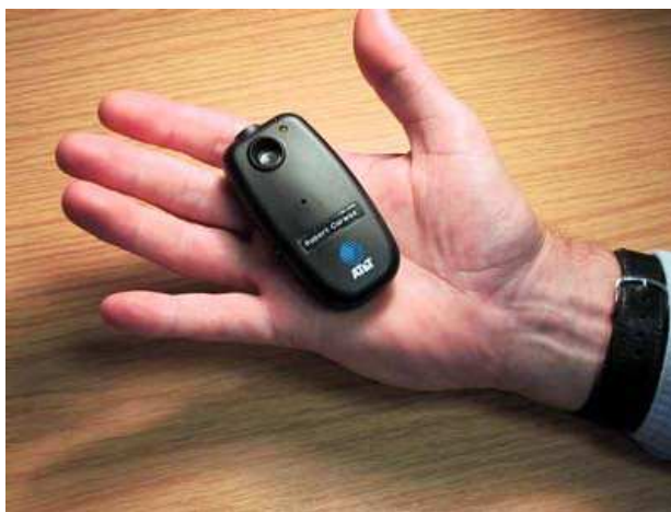
Figure 6: Mobile “Bat” of the At&T Cambridge Active Bat location system. Image courtesy of AT&T Laboratories Cambridge.
