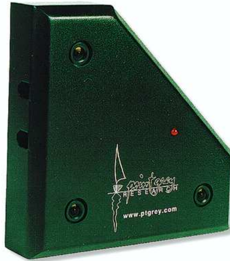
Figure 8: Digiclops color 3D camera, made by Point Grey Research and used by the Microsoft Research Easy Living group to provide stereo-vision positioning in a home environment. Image courtesy of Point Grey Research Inc.
