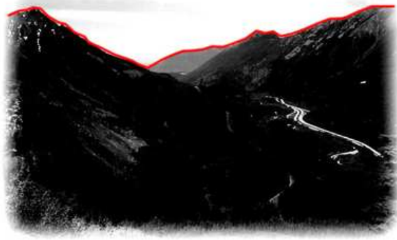
Figure 3: Horizon shapes extracted from a visual scene can be used statically to look up the observer’s location from a prebuilt dataset or dynamically to compute movement of the vehicle mounted camera.
