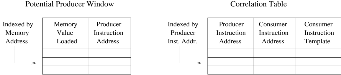
Figure 8. Potential Producer Window (PPW) and Correlation Table (CT) used for detecting linked memory references.
