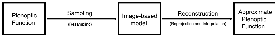
Figure 2: Image-based modeling and rendering pipeline.
