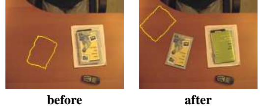
Figure 5: Example of an incorrect transformation with low matching error, due to a uniform background (computed foreground is outlined in both images). Note that in this solution, most pixels in the event region (figure 4(c)) are not transformed onto the event region.
