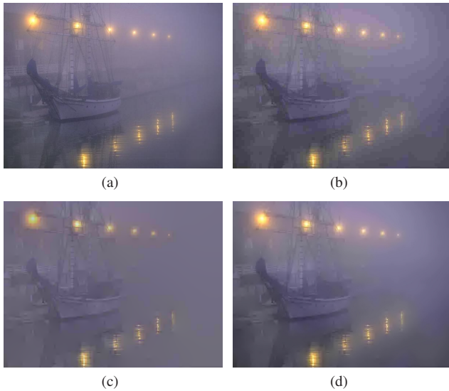
Figure 6: A demonstration of our improvement to Levin’s method for de-blocking images. (a) Original image. (b) Image after compression. (c) De-blocking result using gradient suppression but no data constraints (similar to Levin’s approach); Notice how the highly compressed regions get flattened in appearance. (d) Result produced by our de-blocking method, which uses gradient suppression to reduce blockiness and data constraints to maintain fidelity to the input.
