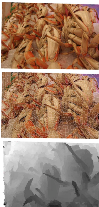
Figure 3 Crab example: the top row shows one of the input images, the middle row is the visualization of its segmentation, and the bottom row is the corresponding depth map.
