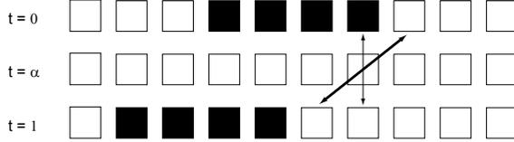
Figure 5: ordering reasoning on the example of fig. 2. At a given intermediate-time pixel, follow each candidate flow forward and backward. Here the diagonal flow will be chosen as the more color-consistent.
