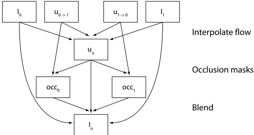
Figure 1: data flow through the three steps of our general approach. Input frames  $I_0$  and  $I_1$ ; forward and backward optical flows  $\vec{u}_{0 \rightarrow 1}$ ,  $\vec{u}_{1 \rightarrow 0}$ ; occlusion masks  $occ_0$ ,  $occ_1$ ; interpolated frame  $I_\alpha$ .
