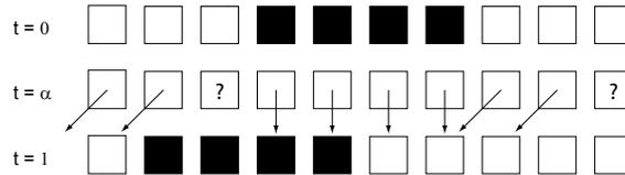
Figure 3: one interpolated flow field we might create for the example in fig. 2, shown pointing forward in time from  $t = \alpha$  but meant to be valid for the entire interval  $t \in [0, 1]$ .
