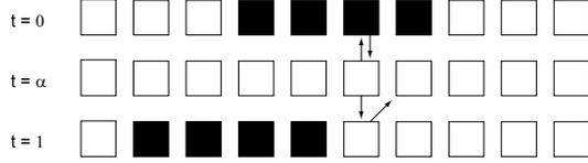
Figure 7: occlusion reasoning on the example of fig. 2. Follow the chosen flow forward and backward from  $t = \alpha$  and compare to the flows at those locations at  $t = 0$  and 1. We determine this pixel to be visible in  $I_0$  and possibly in  $I_1$ .
