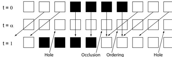
Figure 2: forward splatting demonstrated on a synthetic dataset. Top and bottom rows are  $I_0$  and  $I_1$ . Arrows show the forward flow and which pixel locations it passes through at  $t = \alpha$ . Three types of problem: holes (intermediate-time pixels with no flows through them); ordering (intermediate-time pixels with multiple flows through them); occlusion (multiple flows to the same  $t = 1$  location).
