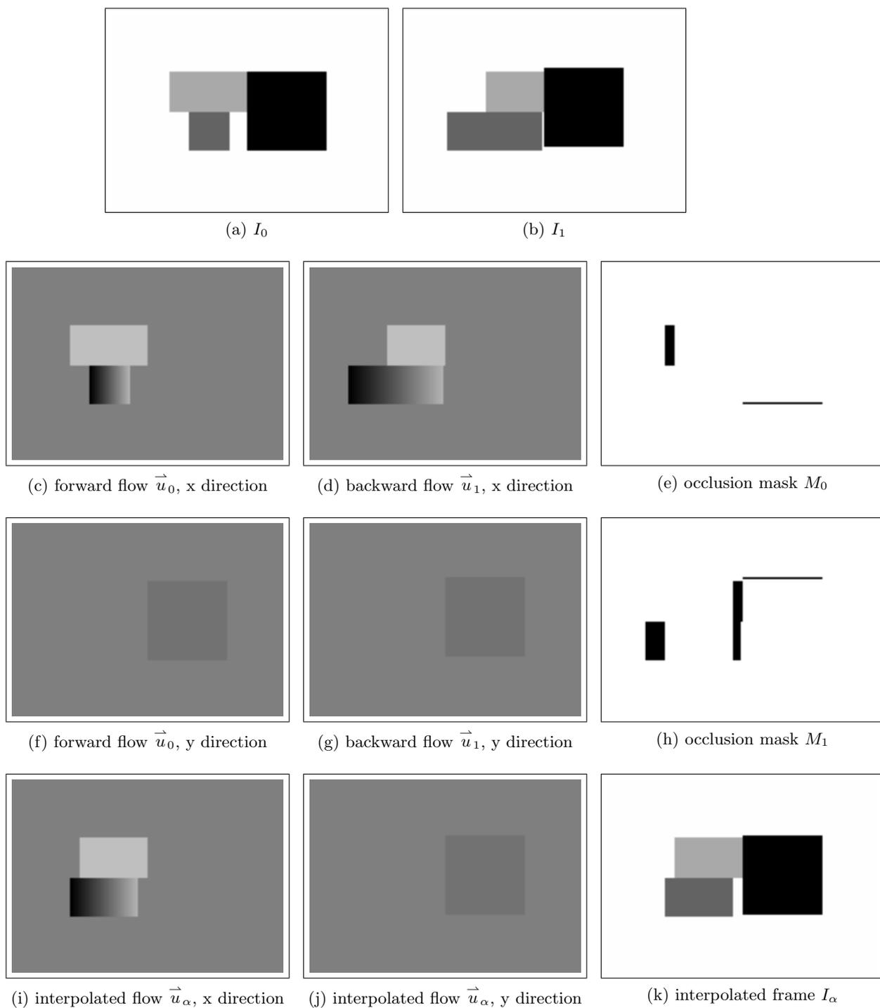
Figure 8: a synthetic example dataset. True motion: the light gray object moves right; the black object moves up; the dark gray object moves left and expands horizontally.
