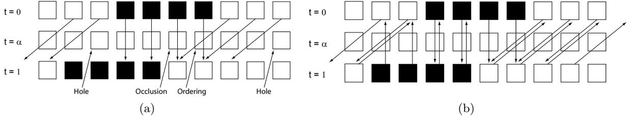
Figure 6: bidirectional splatting reduces holes. (a) forward splatting (fig. 2 repeated); (b) bidirectional splatting.
