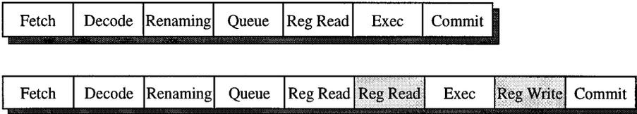
Fig. 3. Comparison of the pipelines for a conventional superscalar processor (top) and the SMT processor's modified pipeline (bottom).
