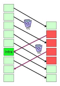
Figure 2: Demonstration of single intra frame recovering from multiple losses. The state of the encoder and decoder are on the left and right respectively. Time advances toward the bottom of the page.
