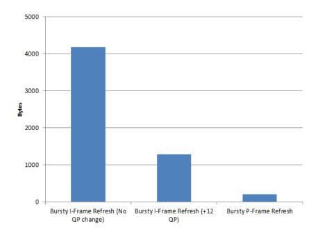
Figure 5: the packet size of a refresh frame for three different cases when the second frame is lost.
