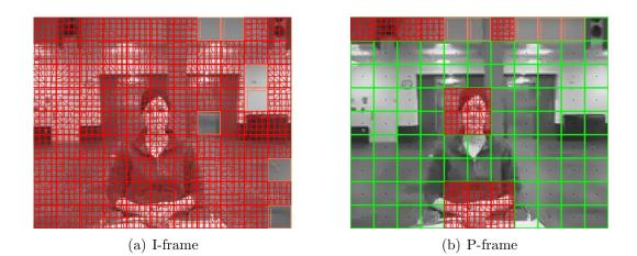
Figure 1: Comparison of number of intra-blocks contained in an I-frame and a P-frame used for refreshing. Intra-blocks are drawn in red and skip-blocks are indicated with green. Most gains will not be as extreme. Note that there are many I-blocks in faces and hands.
