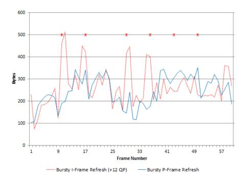
Figure 4: Resulting Packet Size for different recovery techniques on the test sequence. An asterisk indicates the time frames are lost. Note that our target average bit rate is 30 kbps.
