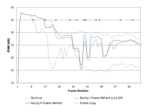
Figure 6: Resulting PSNR for different recovery techniques on the test sequence. An asterisk indicates the time frames are lost. Note that the bursty P-frame refresh recovers more quickly from a loss than adjusted bursty I-frame refresh.
