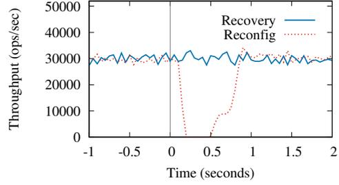
(b) Throughput during a single recovery and re-configuration with wide-area latencies starting at time 0
