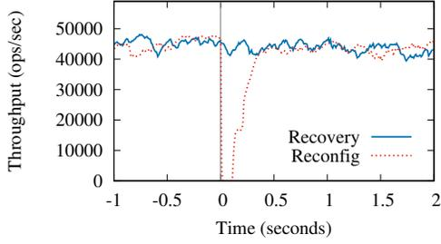
(a) Throughput during a single recovery and re-configuration starting at time 0
